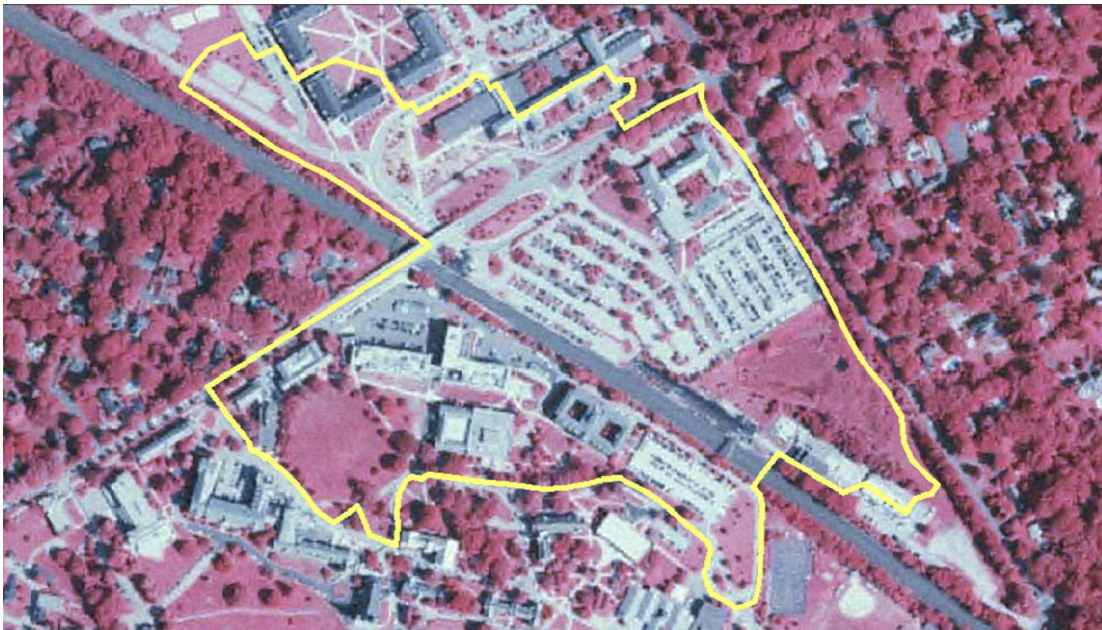
Figure 4. Infrared image of the Villanova University constructed stormwater wetland drainage area (solid line).
