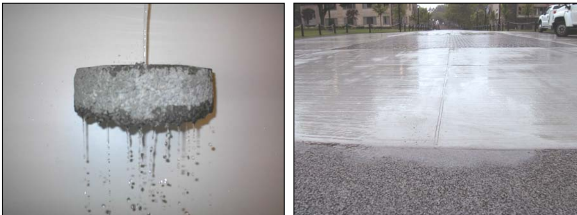
Figure 1.6 Illustration of the Ability of Porous Concrete to Convey Water
